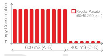
LP LED is the latest release in individual electronic Pulsators. The LEDs provide a visual information about Pulsation status. PWM technology (Puls-Width Modulation) allows to save 40% energy.
